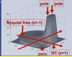
Pole near unit-circle introduces 'peak' in frequency response
